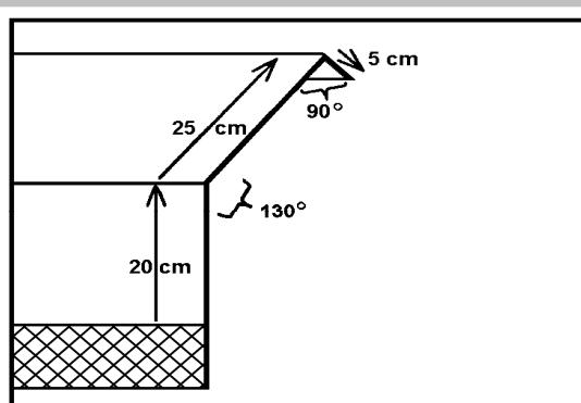
**Figure 3: Overhang for inner fences**
