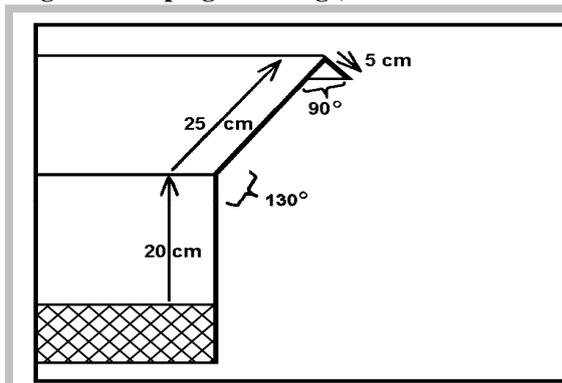
Figure 3: Overhang for inner fences
